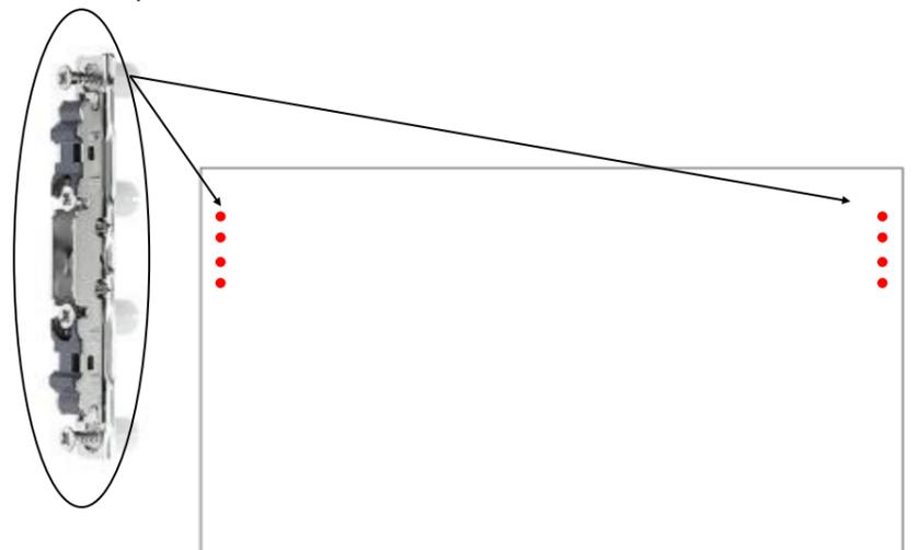
**1 Take the LIFT mechanism** & seat the two locating lugs (small indents) on the two pre-drilled holes.
