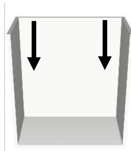
The top & bottom of your carcass are dowelled into the back & the gable so ensure these are correctly located.
