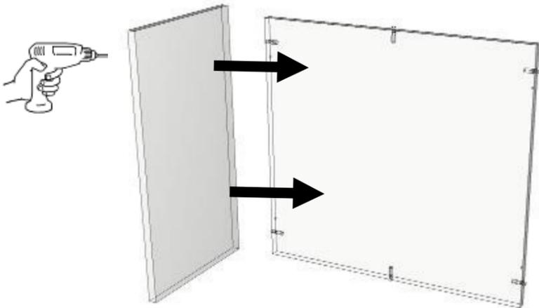
**4 Now place carcass on end.** Insert dowels into the top & bottom ... and insert these into the gable.
