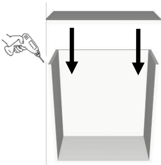
**6 You are now ready to assemble** the LIFT mechanism: .... Open the Aventos Hardware boxes and identify the 2 x Door Mounting plates. These can be screwed to the door by pressing in securely and then screwing the four screws down firmly with a cordless drill. For now place the door to one side.
